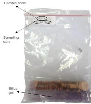
Fig. 3. Wood core in a plastic zip lock bag (12 cm x 20 cm).
